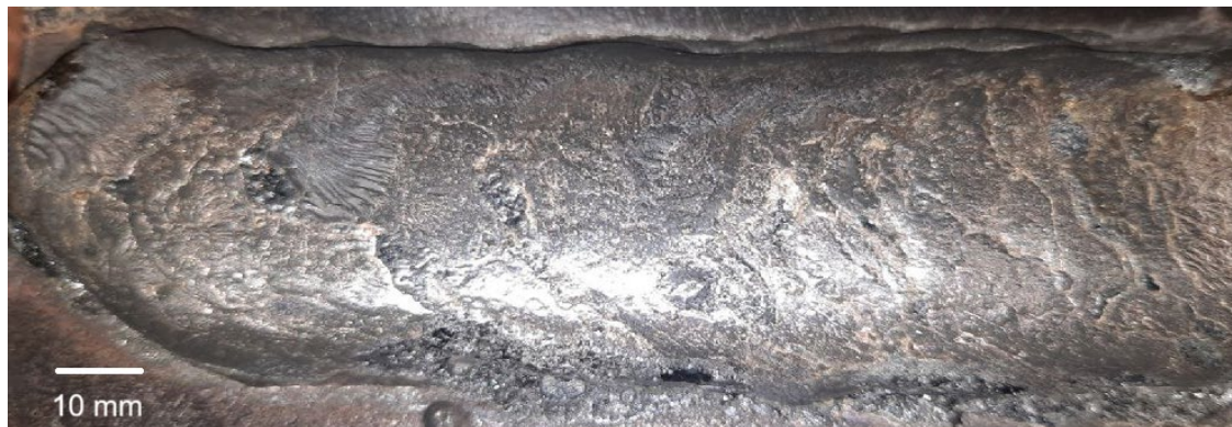
Fig. 2. Cladded by three electrode bundle deposit layer
