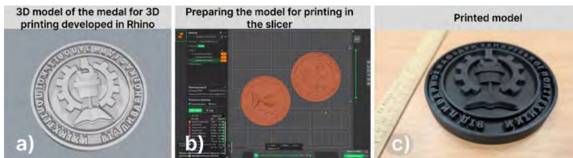
Fig. 1. 3D model of the medal developed in Rhino and preparation for 3D printing in the slicer
