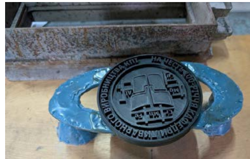
Fig. 2. Hybrid pattern assembly: a 3D-printed PLA master pattern with an attached wax gating system
