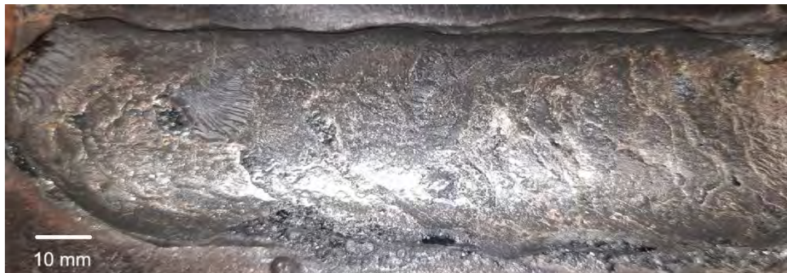
Fig. 2. Cladded by three electrode bundle deposit layer
